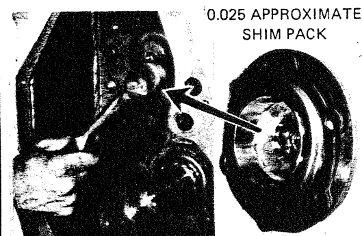
STEP 16. Install approximately 0.025 inch shim pack on left-hand bearing retainer, then install retainer. Tighten capscrews securely. Final torque at this time is not necessary.
